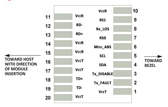
Host PCB SFP+ Pad Assignment Top View
